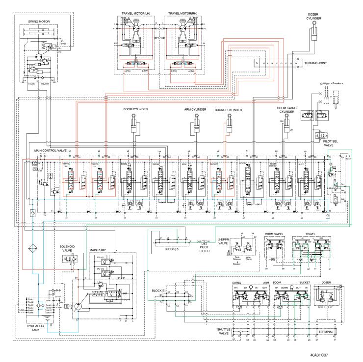
When the arm and travel functions are operated, simultaneously the arm spool and travel spools in the main control valve are moved to the functional position by the pilot oil pressure (a5, b5, a1, b1, a2, b2) from the remote control valve.
