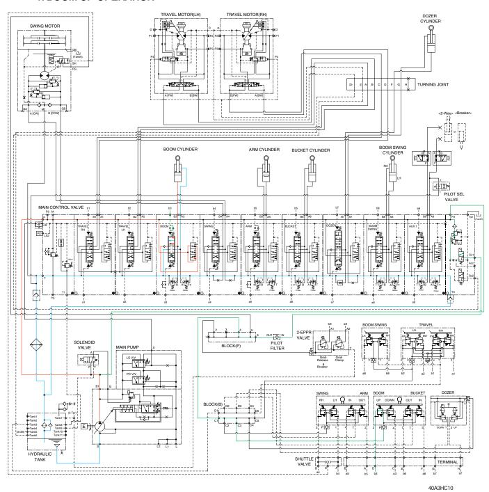
When the right control lever is pulled back, the boom spool in the main control valve is moved to the up position by the pilot oil pressure (b3) from the remote control valve.
