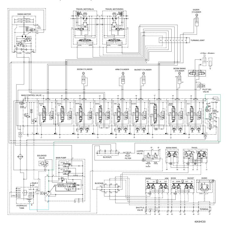
When the lever of the safety solenoid valve is moved downward, oil flows into the remote control valve through solenoid valve and line filter in the main control valve.
