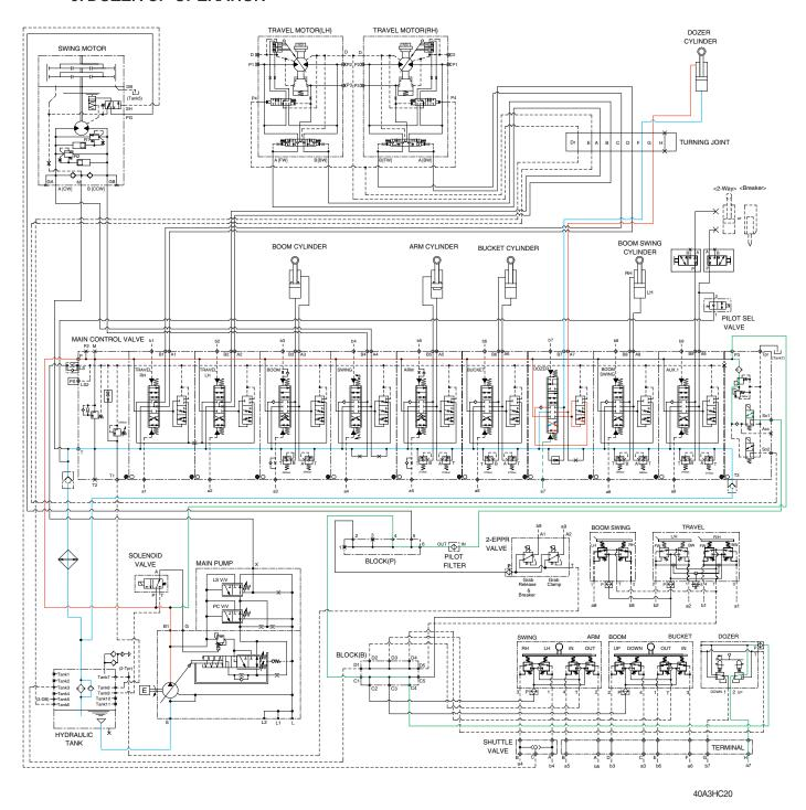
When the dozer control lever is pulled back, the dozer spool in the main control valve is moved to the dozer up position by the pilot oil pressure (a7) from the remote control valve.
