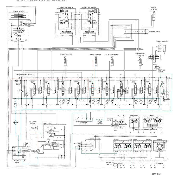
When the left control lever is pushed forward, the arm spool in the main control valve is moved to the roll out position by the pilot oil pressure (b5) from the remote control valve.
