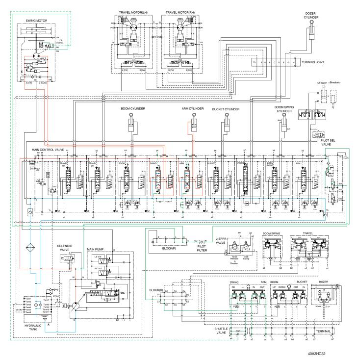
When the swing and arm functions are operated, simultaneously the swing spool and arm spool in the main control valve are moved to the functional position by the pilot oil pressure (a4, b4, a5, b5) from the remote control valve.
