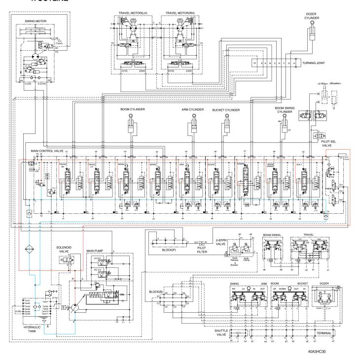
The oil from the main pump flows through the parallel oil passage in the main control valve. Then the oil goes to each actuator and operates them. Check valves and orifices are located on these oil passage in the main control valve. These control the oil from the main pumps so as to correspond to the operation of each actuator and smooth the combined operation.
