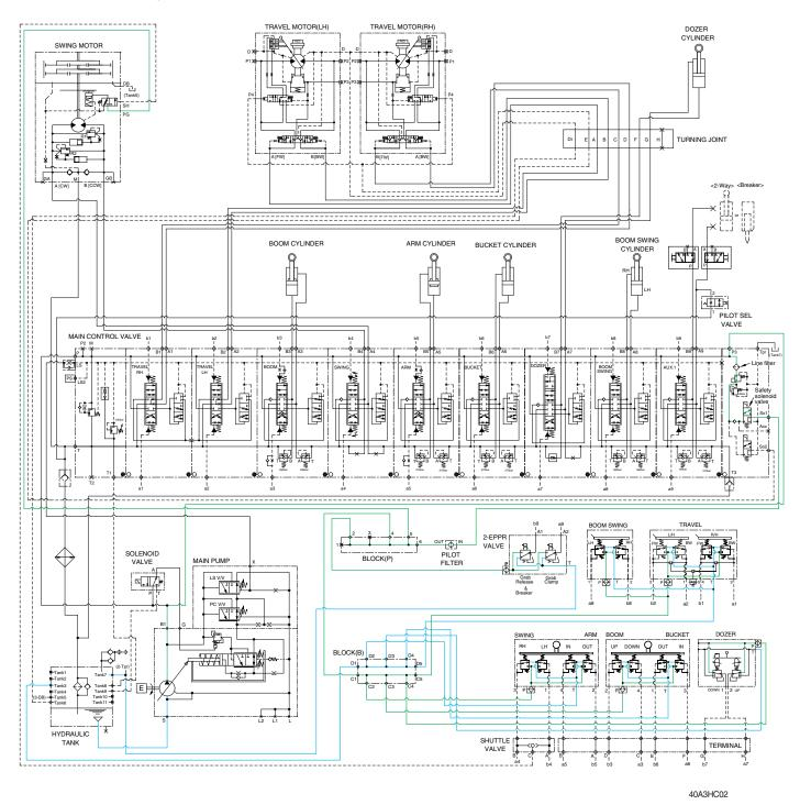
The main pump receive oil from the hydraulic tank. The discharged oil from the main pump flows to the safety solenoid valve through the line filter. The oil is filtered by the line filter. The pilot relief valve is provided in the main control valve for limiting the pilot circuit pressure.
