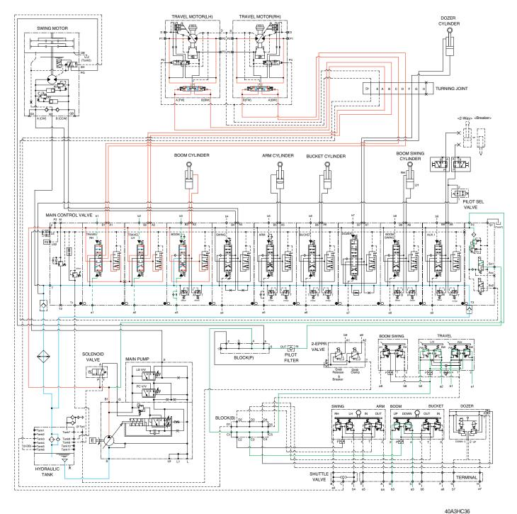
When the boom and travel functions are operated, simultaneously the boom spool and travel spools in the main control valve are moved to the functional position by the pilot oil pressure (a3, b3, a1,b1, a2, b2) from the remote control valve.
