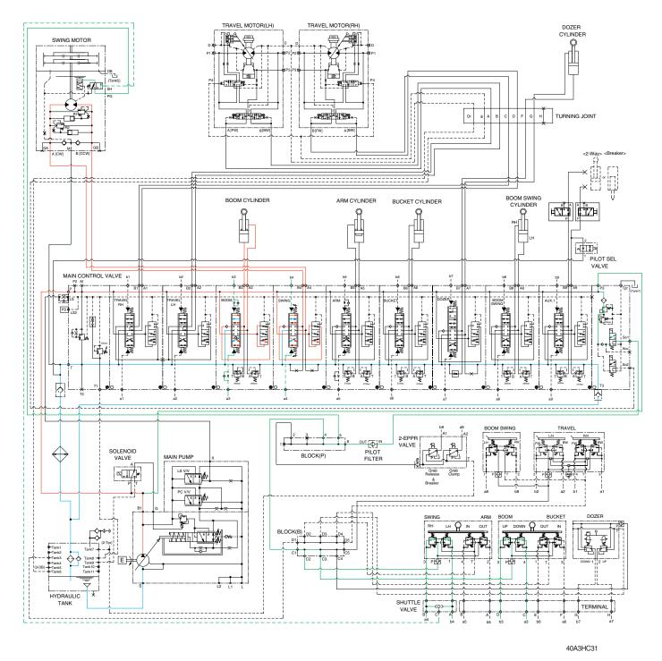
When the swing and boom functions are operated, simultaneously the swing spool and boom spool in the main control valve are moved to the functional position by the pilot oil pressure (a4, b4, a3, b3) from the remote control valve.
