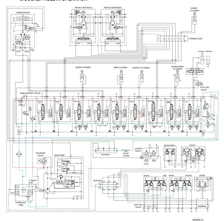
When the right control lever is pulled left, the bucket spool in the main control valve is moved to the roll in position by the pilot oil pressure (a6) from the remote control valve.
