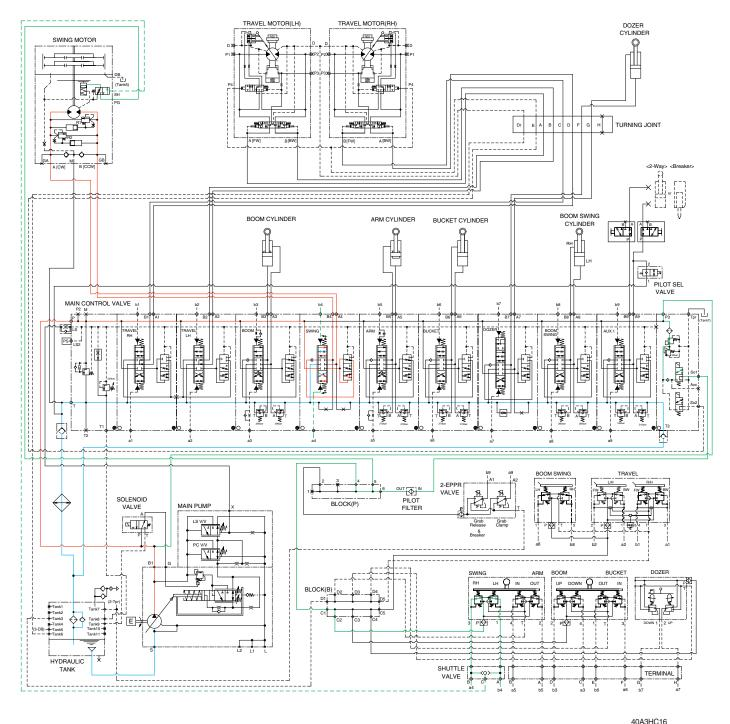
When the left control lever is pushed left or right, the swing spool in the main control valve is moved to the left or right swing position by the pilot oil pressure (a4, b4) from the remote control valve.
