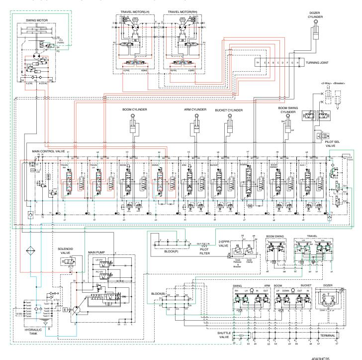
When the swing and travel functions are operated, simultaneously the swing spool and travel spools in the main control valve are moved to the functional position by the pilot oil pressure (a4, b4, a1, b1, a2, b2) from the remote control valve.
