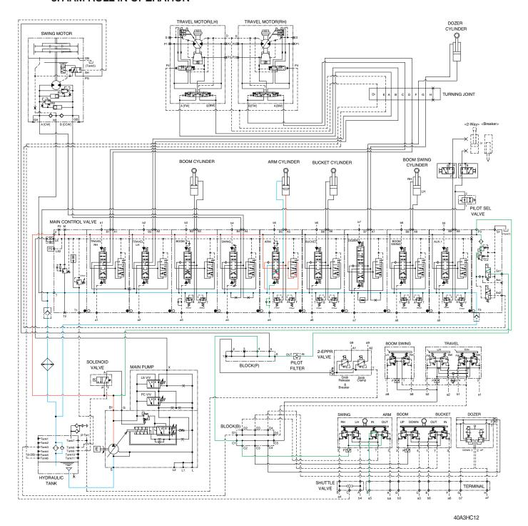
When the left control lever is pulled back, the arm spool in the main control valve is moved the to roll in position by the pilot oil pressure (a5) from the remote control valve.
