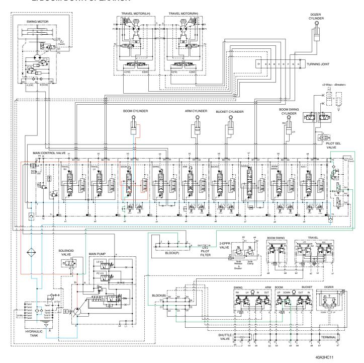
When the right control lever is pushed forward, the boom spool in the main control valve is moved to the down position by the pilot oil pressure (a3) from the remote control valve.
